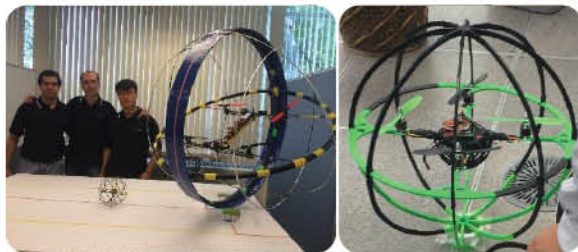
Skypersonic team at Lawrence Tech University and some different prototypes of sphere-copter
