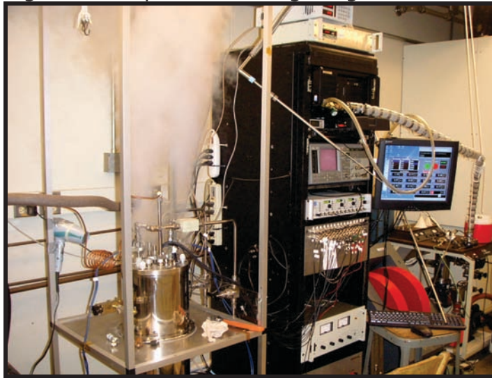
Fig. 2 Magnet testing in temperatures between 4.2 K and 36 K
